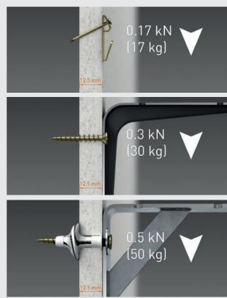
Fixing and maximum load-holding strengths are shown above, all into a single layer of 12.5 mm fermacell<sup>®</sup> board without plywood pattressing. N.B safety factor of 2.
