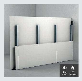
**System specification: 1S15** 12.5 mm fermacell® board either side of 75 mm steel stud.
