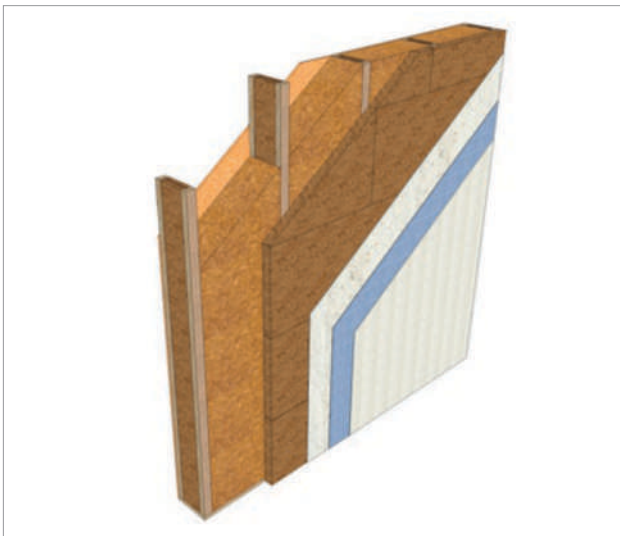
Timber frame with no external board material
